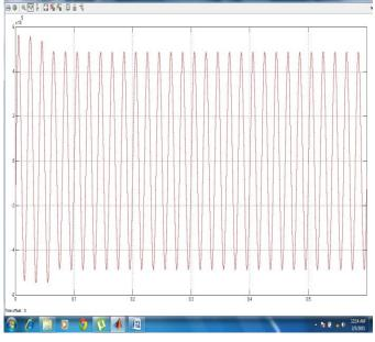
Figure- 9 500KV Bus Bar Voltage during Phase-Ground fault.
