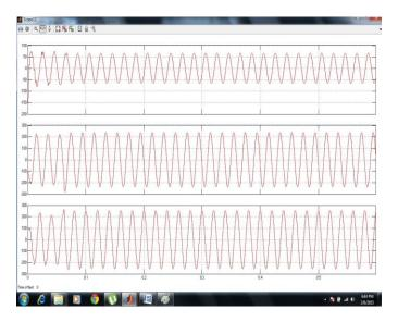
Figure- 12 132 KV Transmission Lines current during 500KV line faults.
